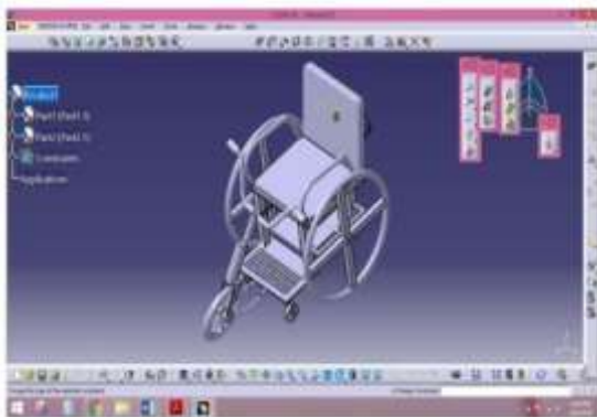
Fig.7 CAD model of the wheelchair
